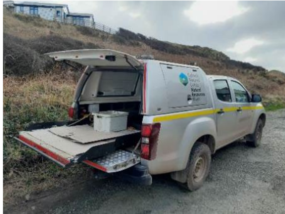
Figure 5.5 Isuzu pickup truck with sliding boot tray.
